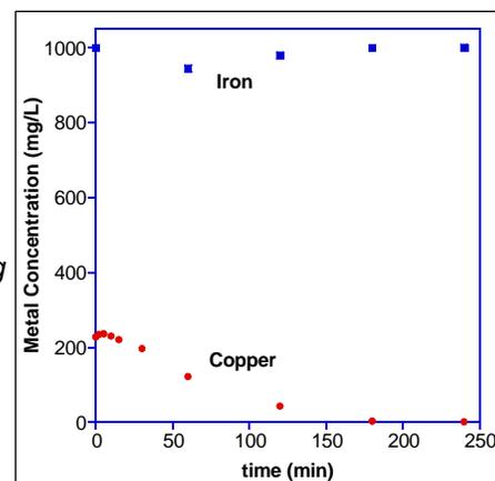
*Copper removal from a mixture of copper and iron, pH 2.3 H<sub>2</sub>SO<sub>4</sub> electrolyte, batch process.*
