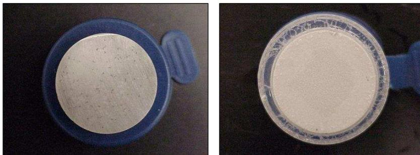
**Figure 4.** Left: un-anodized AZ61 shows corrosion pitting after only 2 hours immersed in a 1.0 M MgCl<sub>2</sub> salt bath. Right: AZ61 anodized using Eltron's process shows no corrosion after 168 hours immersed in a 1.0 M MgCl<sub>2</sub> salt bath.
