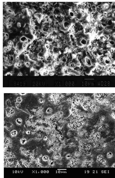
**Figure 1.** 1000X SEM images of the surfaces of anodized ZE41 magnesium alloy. Top: Coating produced by the Tagnite process.\* Bottom: Coating produced by Eltron's low-cost process.
