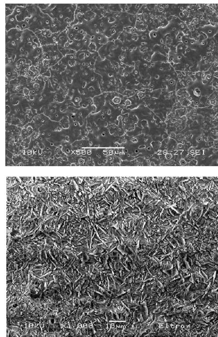
**Figure 2.** Anodized magnesium alloy coatings. Top: Amorphous coating. Bottom: Crystalline coating.
