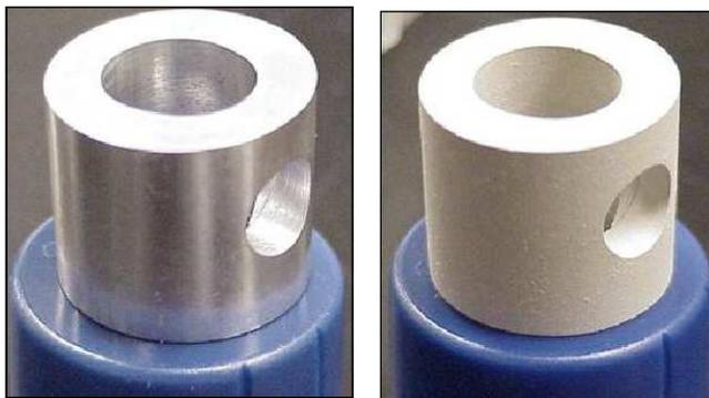
**Figure 3.** Left: AZ61 alloy before anodization. Right: AZ61 alloy after anodization.
