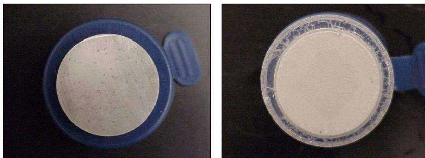
Figure 4. Left: un-anodized AZ61 shows corrosion pitting after only 2 hours immersed in a 1.0 M MgCl 2 salt bath. Right: AZ61 anodized using Eltron's process shows no corrosion after 168 hours immersed in a 1.0 M MgCl 2 salt bath.
