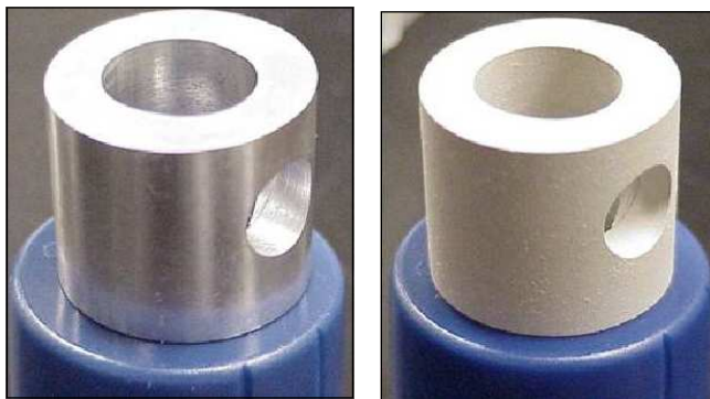
Figure 3. Left: AZ61 alloy before anodization. Right: AZ61 alloy after anodization.
