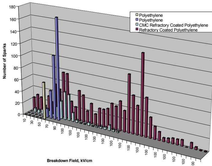
**Figure 2.** Tracking resistance of refractory coated HDPE cylindrical insulators compared to uncoated polyethylene. Refractory coated HDPE can withstand over 1000 more flash over sparks than uncoated polyethylene.
