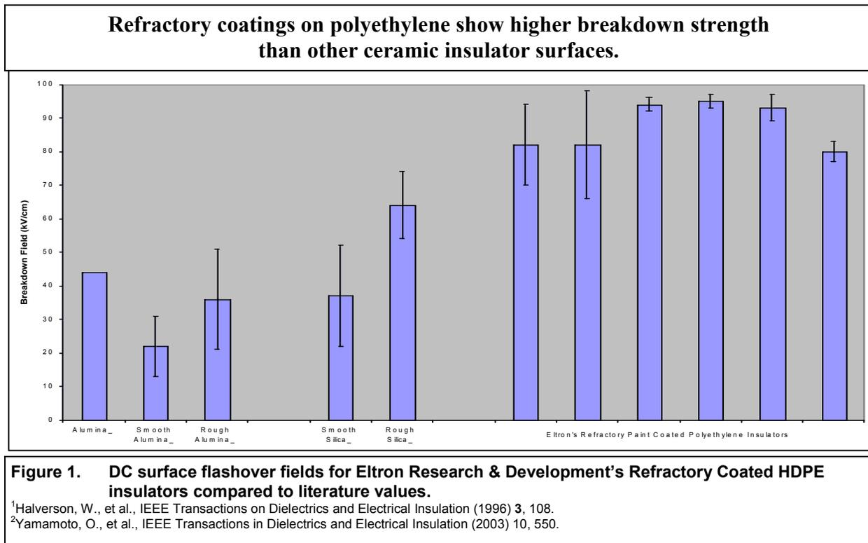
**Figure 1** shows the surface flashover performance in vacuum of Eltron's refractory coated plastic insulators, compared to insulators made of refractory ceramics such as alumina and silica. Eltron's coatings exceeded the surface flashover field of common electrically-insulating ceramics. In addition, the refractory coatings have excellent high-temperature resistance (>1000°C) compared to polyethylene (~120°C).
