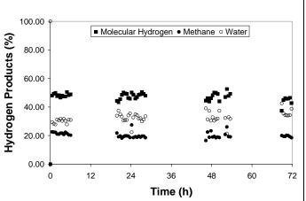
Eltron catalysts produce hydrogen and carbon monoxide with good efficiency from ULSD fuels throughout 72 hour tests with no drop in performance. Tests were conducted with 20% excess oxygen relative to stoichiometric partial oxidation.
