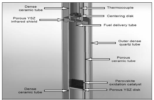
This 3D model of a single-tube reactor is similar to the multi-tube reactor design Eltron has produced for the generation of synthesis gas. When coupled with a solid-oxide fuel cell, the multi-tube design will yield sufficient synthesis gas to generate 5 kW of-clean electricity.
