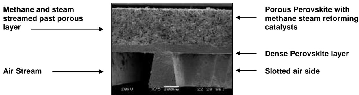
**Figure 1. A cross section of a planar oxygen transport membrane. The top, porous layer supports steam reforming catalysts. The middle, dense layer allows diffusion only of oxygen anions and gives the membrane essentially 100 % selectivity for oxygen. The lower slotted region is used for mechanical support in resisting differential pressures of 250 psi.**
