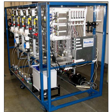
H 2 O 2 /PAA Water Treatment System Developed at Eltron Water Systems
