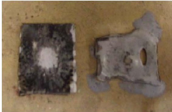
Figure 4: Refractory paint coated square (left) and uncoated square (right) of high density polyethylene after exposure to direct flame of a propane torch for 20 seconds, at a distance of 2.5 cm (1 in.).
