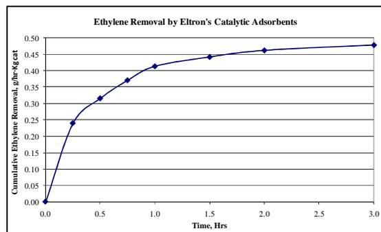
Figure 1. Data demonstrating ethylene removal activity for Eltron's catalytic adsorbent. Experiments were conducted at 2°C with 20 ppm ethylene and a space velocity of 18,000 hr<sup>-1</sup>.
