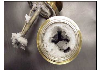
Figure 1. Photograph of reactor containing FTS wax after reaction of simulated syngas over Eltron's patented catalyst.
