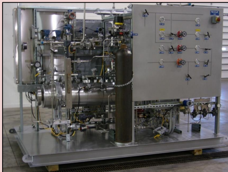
Eltron's Hydrogen Membrane project continues to make progress. In the picture above is the pilot 12-lb/day unit that was designed and fabricated by Continental Technologies and is now located at Eltron's partner Eastman Chemicals in Tennessee.
