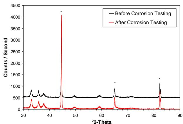
**Figure 2.** X-ray diffraction patterns for AlN coated 1018 carbon steel before (top) and after (bottom) corrosion testing. An asterisk indicates diffraction peaks corresponding to iron; unlabelled peaks correspond to AlN.
