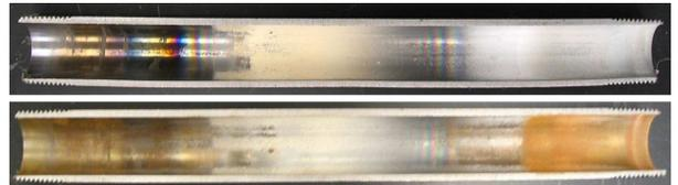
*Cutaway of mild steel pipe following AlN deposition. The top image shows the pipe immediately after deposition. The bottom image shows the effects after six months of testing. Note that the center of the pipe, where the coating was applied, is free of any corrosion.*
